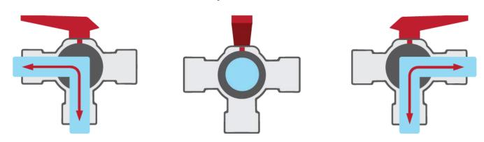
Vertical type L-pattern flow three-way ball valves have two possible flow paths and two possible off positions.
