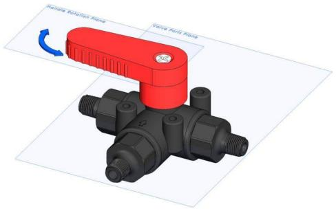
The front view of another common style of three-way ball valve. It has a handle that rotates at a right angle to the valve ports plane. These are also called vertical version, vertical type, vertical ported, upright and upright tee valves.
