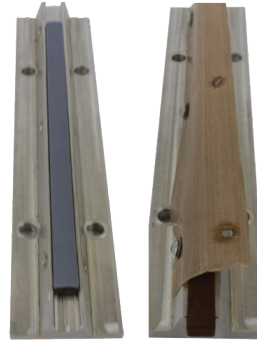
Teflon™ bonded silicone heat seal tool (left)
